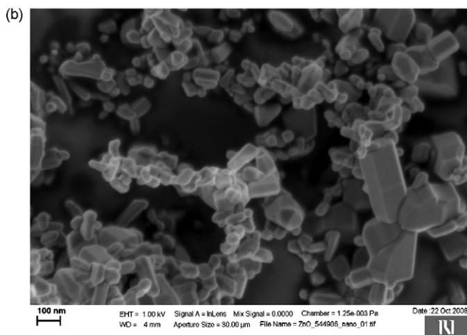
Photo 3. Scanning electron micrograph of nanosized ZnO under low (a) and high (b) magnification.
