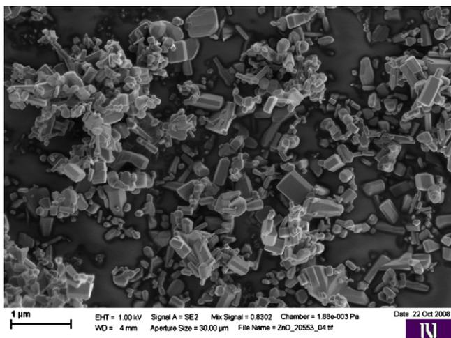
Photo 2. Scanning electron micrograph of ZnO macropowder.
