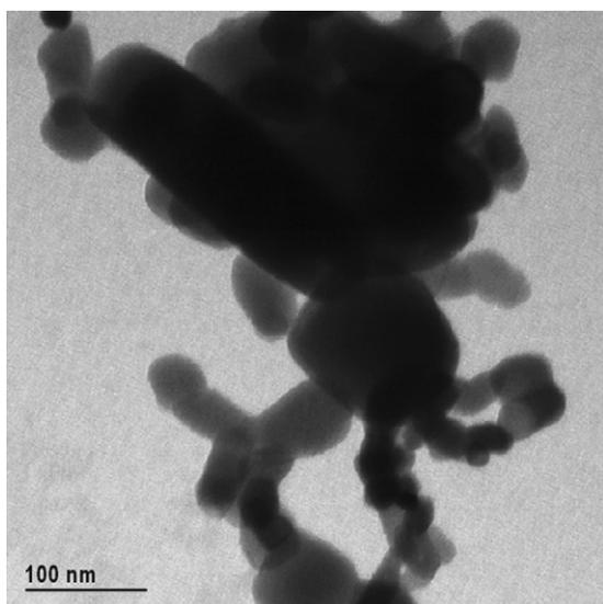
Photo 1. Transmission electron micrograph of nanosized ZnO.
